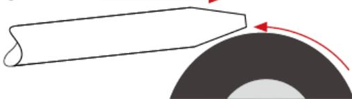
don't grind across the grinding wheel
